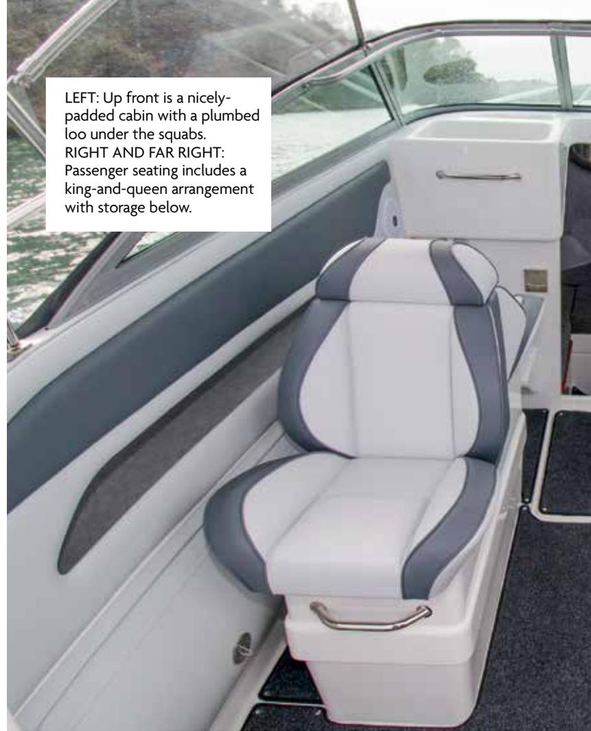
are fully-upholstered, well-protected by the smart black canvas top on sturdy stainless steel supports. The passenger side seat is a king-and-queen arrangement which swings up as one unit to reveal a large storage locker. Under the skipper's seat is a small fridge, and a hatch in the deck between the seats hides a wet storage area.
