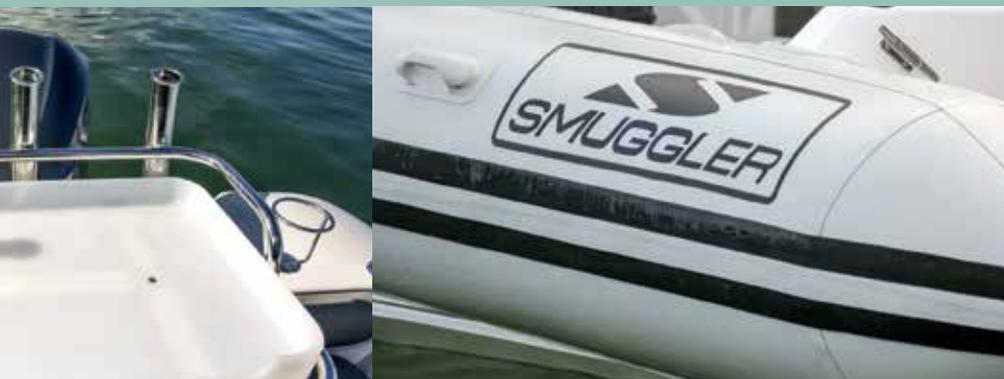
platform on either side and a wide boarding ladder on the port side. Unlike many RIBs, the boarding platforms extend almost to the end of the tubes so climbing aboard is easy. Although there is no step-through on the transom, it's an easy matter to clamber over using the stern seats as a step.
