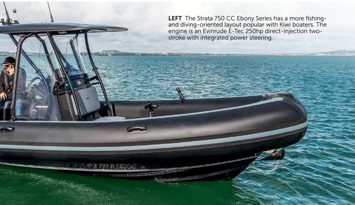
**LEFT** The Strata 750 CC Ebony Series has a more fishing- and diving-oriented layout popular with Kiwi boaters. The engine is an Evinrude E-Tec 250hp direct-injection two-stroke with integrated power steering.
