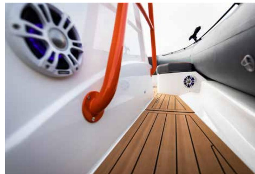
The hardtop is a vacuum foam composite construction which maintains the strength but also keeps the weight to a minimum, so it doesn’t effect the balance and handling of the boat. The bright orange 50mm support keeps everything rigid, with the top sections removeable should you have a storage issue or want to get the boat into a container. The Strata 900 is also available with a full cabin or a cabin with open bow cockpit.
